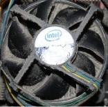
Using a can of compressed air, blow out as much dirt and debris from inside the computer. Pay particular attention to the heat sink and fan (shown to the left), try and blow out as much of the dirt ctuck in
